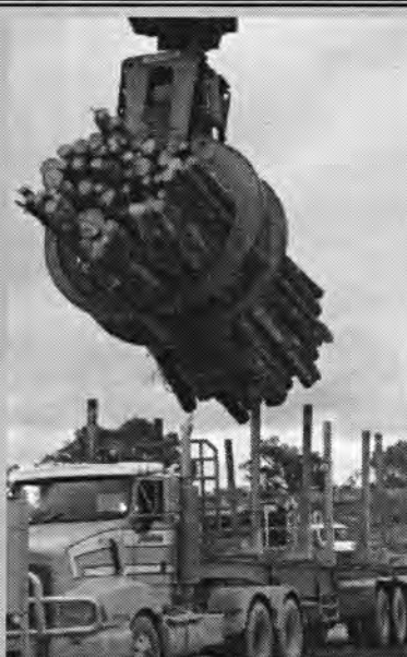
Grapple 'grabs' one truck bay at a time; capacity: 35-40 tonnes.
